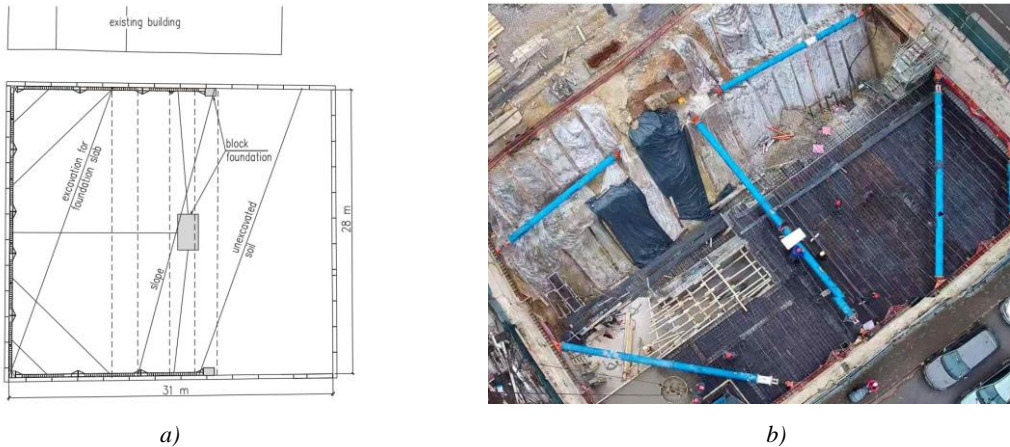
Figure 2. Excavation plan during stage 1 a) plan; b) section
