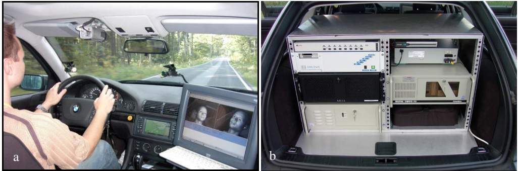
Figure 5. Eye-tracking system in the measurement vehicle (a) and central computer in the trunk (b)
