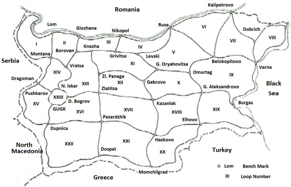
Figure 1. Scheme of the Third Precise Levelling Network of Bulgaria
