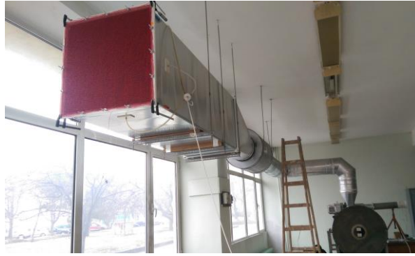
Figure 2. Installed cladding specimen prior to testing
