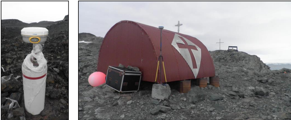
Figure 5. a) Base receiver set up on the permanent GNSS marker KOH2; b) Rover receiver measuring the chapel's roof corners for TLS data georeferencing
