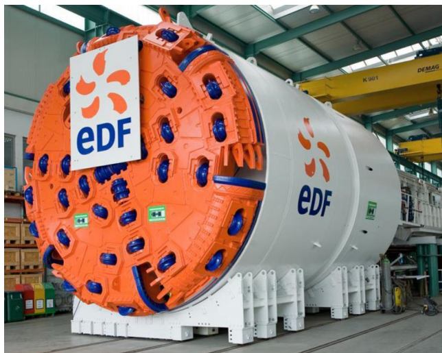
Figure 5. Mixshield (Ø 6,11 m) applied to construct the undersea tunnel
