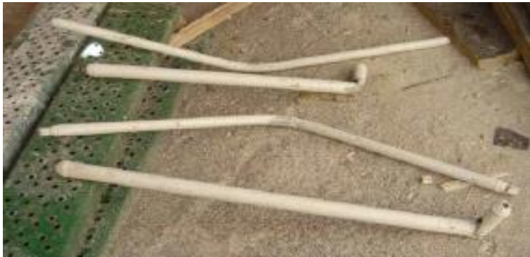
Figure 6. Buckled bars of the structure
