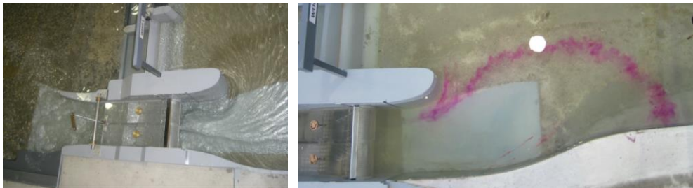
Fig. 17. Flood water discharge through the new turbine weir bay with different left retaining wall designs
