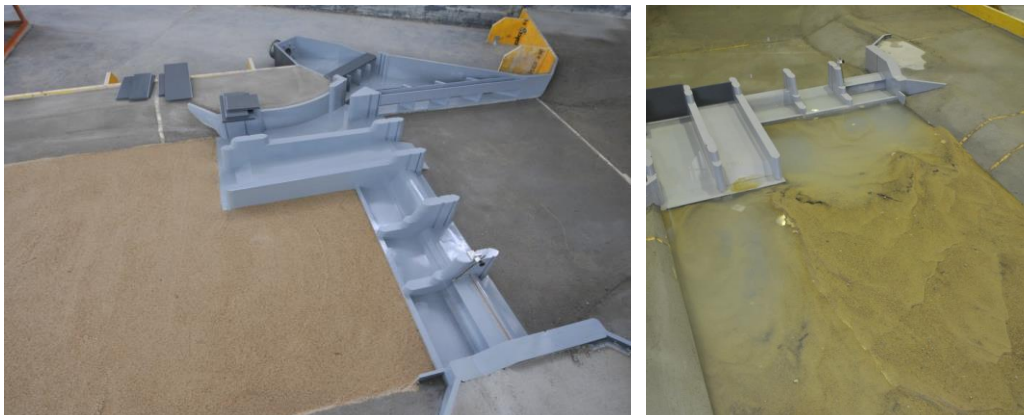
Fig. 13. Downstream region before and after tests with mobile riverbed
