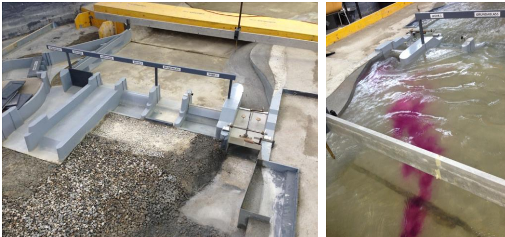
Fig. 19. Downstream view of the final model, flushing during a flood water discharge
