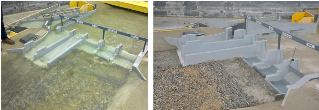
Fig. 14. Scour protection with second stilling basin, heightened end sill of the sluice bay, riprap protection of riverbed; weir bays discharging flood water, downstream region after flood discharges
