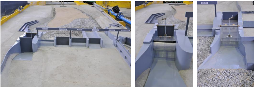
Fig. 15. Upstream and downstream view of the original model with the additional left weir bay
