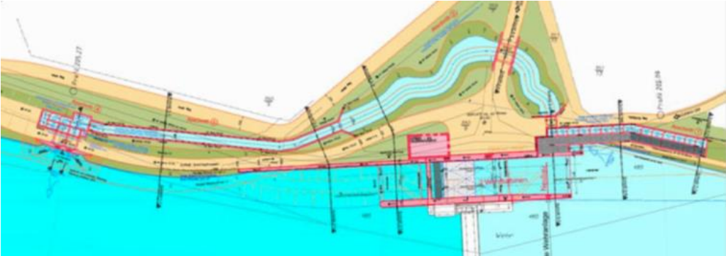
Fig. 7. Layout of the new weir bay with powerhouse module and new fish passage (source: VERBUND)
