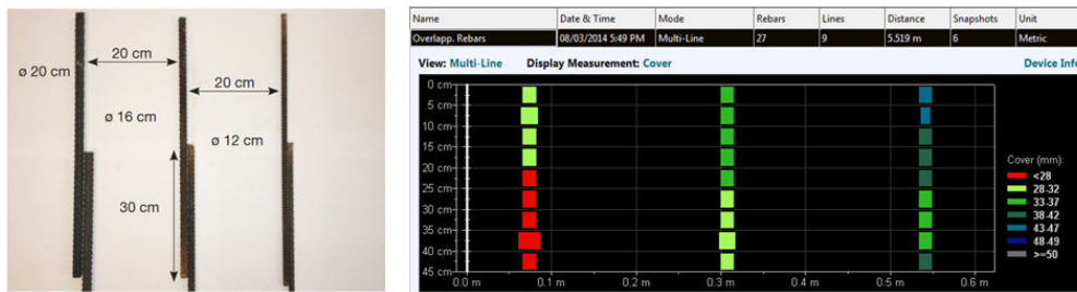
Figure 3. Overlapping rebar arrangement and cover measurement made with Profometer PM-650
