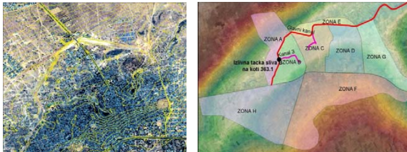
Figure 6. Contour line on the basis of DMT (left) and generated catchments (right)
